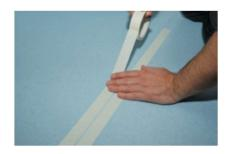
First seal the joints along the car. After the cold weld has cured, seal the seams across the car if applicable. To do so, the 1-component cold weld is spread into the joints without leaving any gaps until a small bulge develops above the seam.
