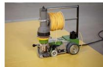
The processing temperature is 350-400° C. When using a welding machine to process the hot welding rod, set the speed to 2 linear metres/minute. The operating speed and temperature can be set on most welding machine.
