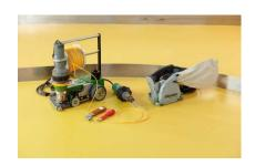
The joints are milled out or cut open centrically with an electric milling machine or the joint cutter.
