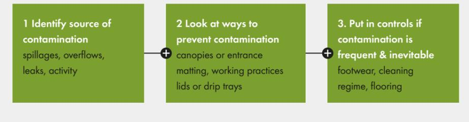
HSE provide a free, online Slips Assessment Tool (HSE SAT tool) to assess the slip potential of surfaces and potential remedies.
