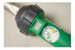
**6.** If the temperature cannot be set, adjust the operating speed accordingly.
